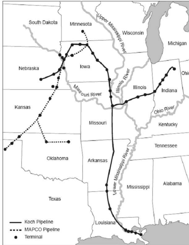
Figure 13. Extant USA liquid \text{NH}_3 pipeline and storage terminal network, handling ~12-15 MMT per year, primarily for N-fertilizer, of which ~60% is imported.
